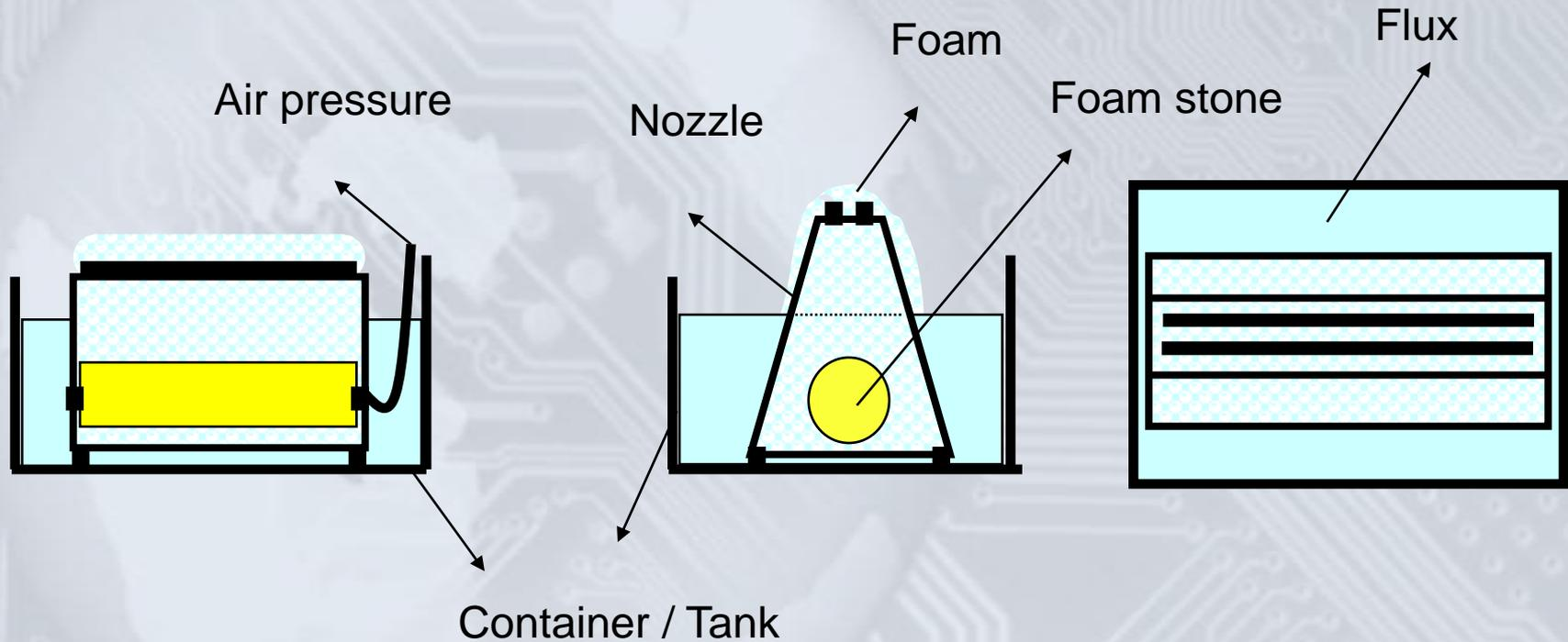
**Materials:** For the flux tank and nozzle, preferably stainless steel or HDPE.
