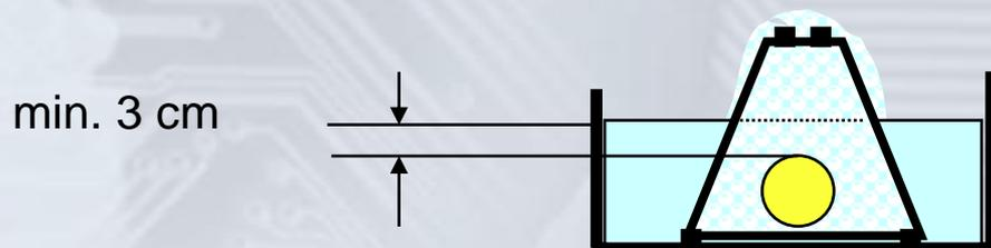
**Air pressure:** As the air passes through the flux, an oil and water separator are necessary. Otherwise the flux can be polluted. Raise pressure until a nice and uniform foam is formed
